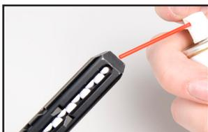
Add a few drops of silicone oil on the BBs located in the BB loading hole. Reinsert the magazine into the gun.
